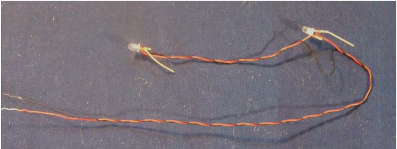
Length of wire with LEDs installed. Keep leads spread apart to avoid a short circuit!
